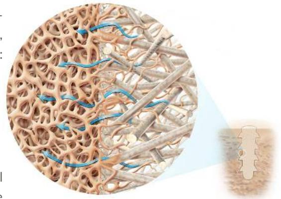
**Figure 1:** Illustration of OSSIOfiber (right) and bone (left) hybrid integration mechanism
