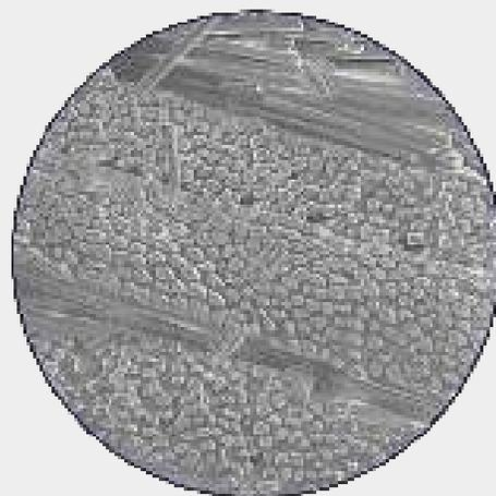
**Figure 5:** Oriented fiber layers as seen in a SEM image of an implant cross-section<sup>9</sup>
