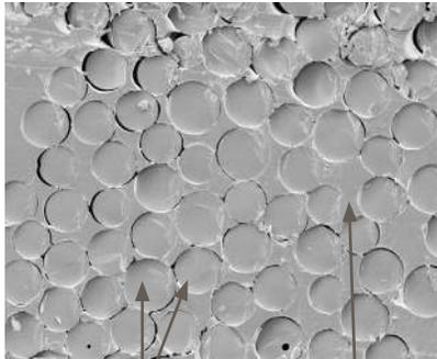
**Figure 3:** Scanning Electron Microscope (SEM) cross-section of OSSIOfiber, highlighting both material components.<sup>9</sup>
